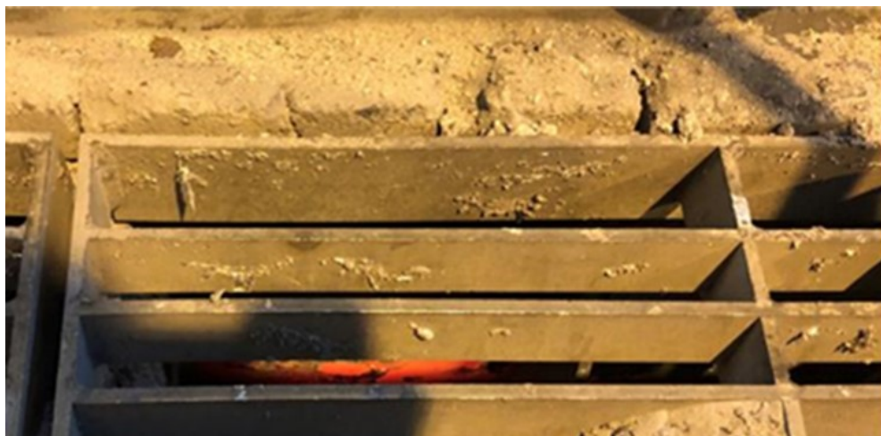
Figure 5. Red spot on the shell of a booster cell in 2021 at AAR-AP60.
